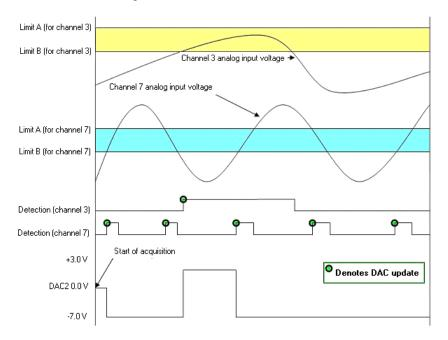
Figure 29. Using two criteria to control an output\*
